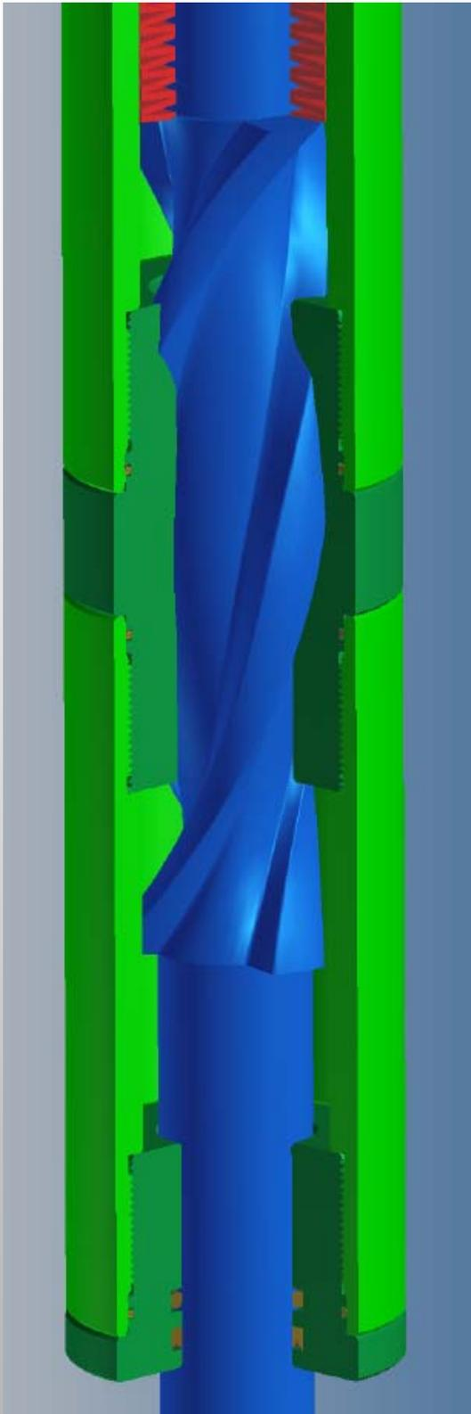
The red conical or Belleville springs are stacked in series or parallel to provide the load rate desired for the job to be done.
