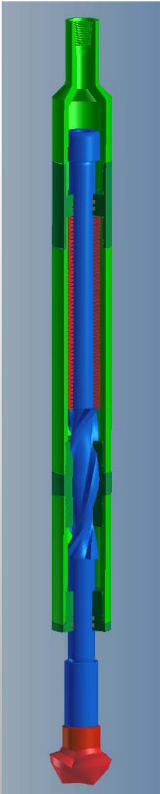
The **CTS TOCA Torque Control Assembly** is designed to prevent over-torquing a drill bit during remediation or virgin drilling operations by **automatically retracting to unload the bit** when a torque obstruction is seen.
